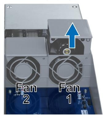
2 Prepare a new fan, align the arrow to point at the back panel as illustrated below, and insert it back into the fan slot.
