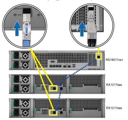
**2** Connect one end of the power cord(s) to the power port of RX1217sas, and the other to the power outlet(s). RX1217sas will automatically power on once the power cords are correctly connected.
