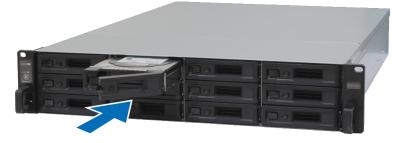
Note: Make sure the tray is pushed in all the way. Otherwise, the drive might not be able to function properly.
