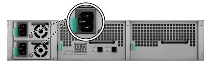
*Note:* Your RX1217sas comes equipped with a redundant power supply system, allowing two power cords to be connected. The system may be powered on with only one power cord, but we recommend using two power cords to avoid unexpected power failures.
